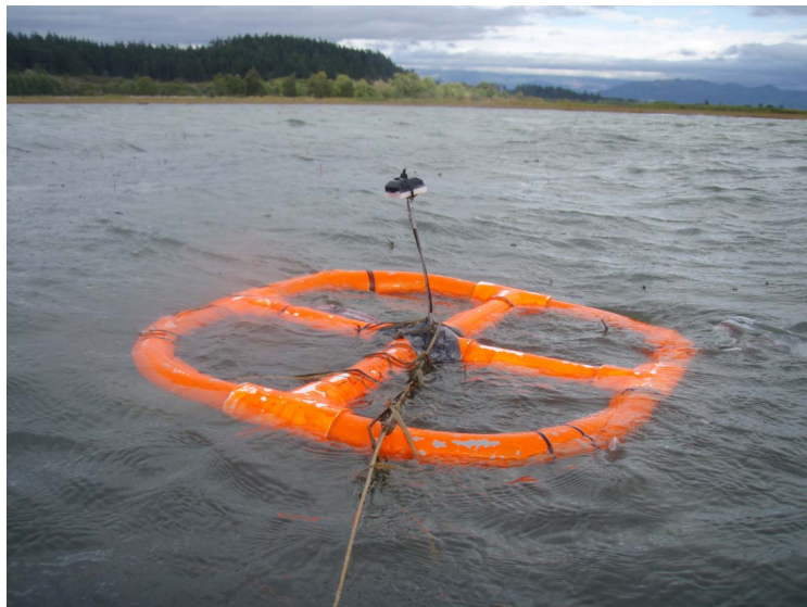
Figure 3: A surface drifter designed to operate in very shallow tidal flats environments. Drifters were drogued to a depth of 30cm, and were mounted with GPS loggers to measure drifter locations, ADCPs to measure the velocity shear beneath the drifters, and thermisters to measure water temperatures.
