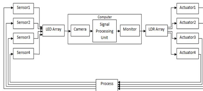
Figure 4: Block Diagram Representation of Computer Interfacing for MIMO System
