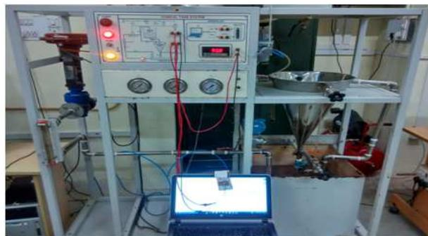
Figure 9: Real Time Implementation and Testing of Computer SISO Interface for Conical Tank System
