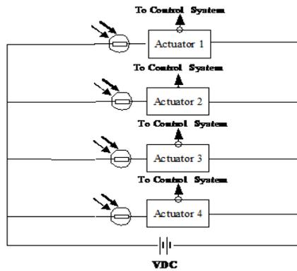
Figure 6: Receiver Circuit for MIMO
