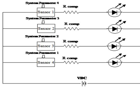
Figure 5: Transmitter Circuit for MIMO
