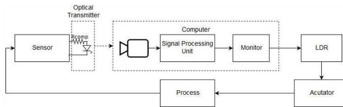
**Figure 1: Block Diagram Representation of Computer Interfacing for SISO System**
