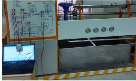
**Figure 10: Real Time Implementation and Testing of Computer MIMO Interface for Heat Exchanger System**
